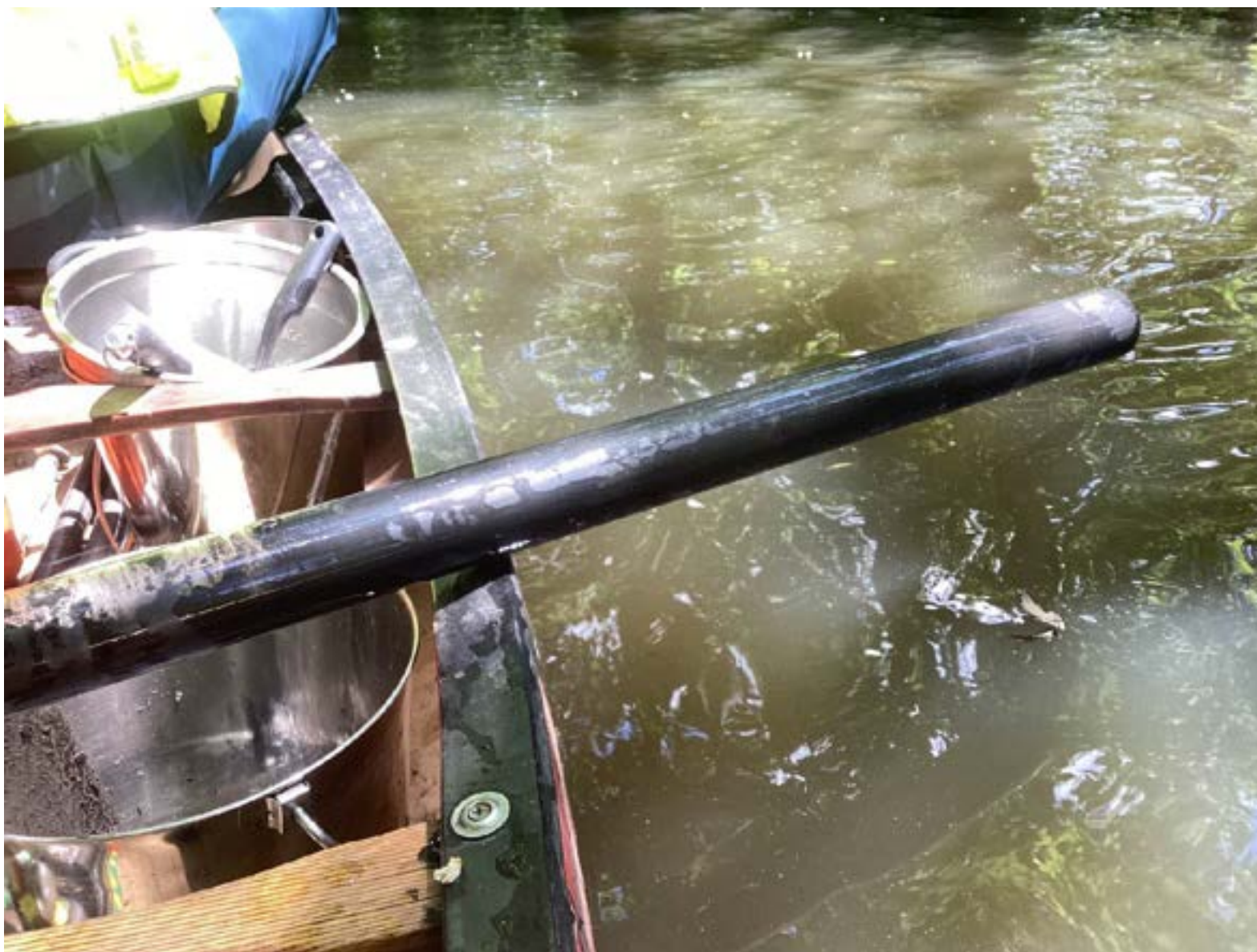
Figure 9. Reach B. Sediment core extracted for Sample AB3.
