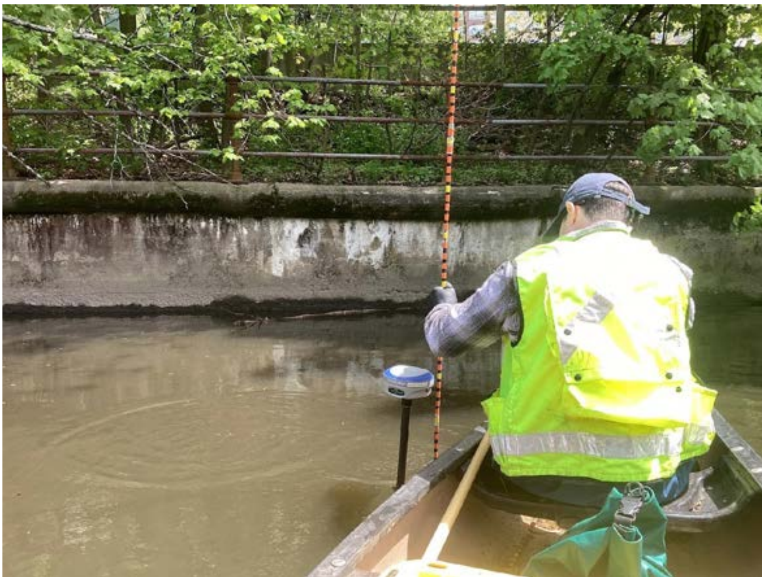
Figure 3. Reach C, looking toward river right. Measuring depth to refusal and sediment thickness using the RTK-GPS and probing rod.
