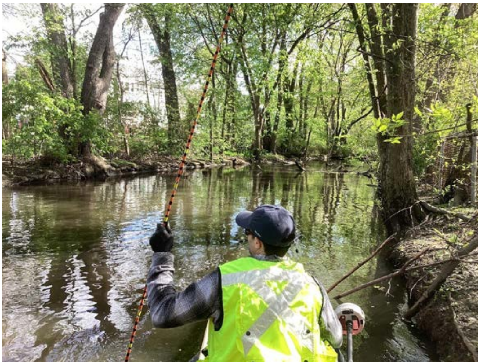
Figure 1. Reach A, looking downstream. Measuring the depth to refusal in the channel using a flexible probing rod.
