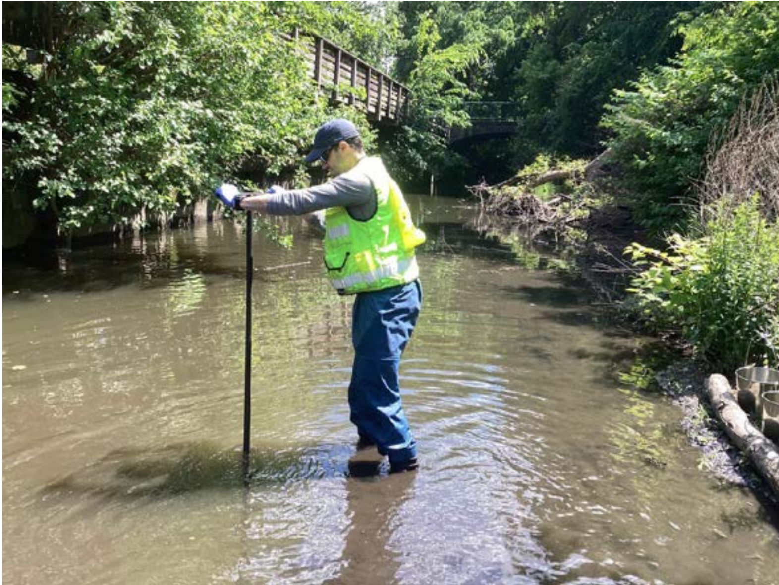
Figure 5. Reach D, looking upstream. Collecting sediment for Sample AB6 using sediment coring tools.
